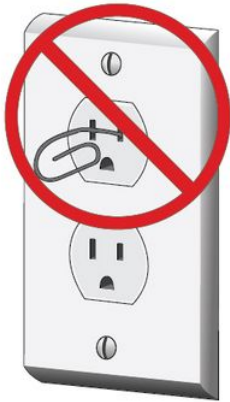
tamper-resistant receptacles won't allow paperclips, keys, etc. into either the hot or neutral slot
